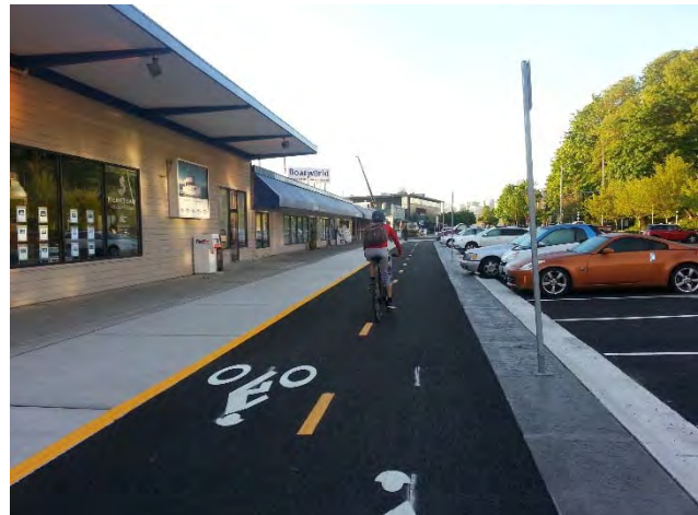
LEFT: Figure 4. Example showing bike/pedestrian symbols in shared travel way (Portland)
